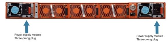
**Figure 2** Connecting AC Power (GigaVUE-HC1)
